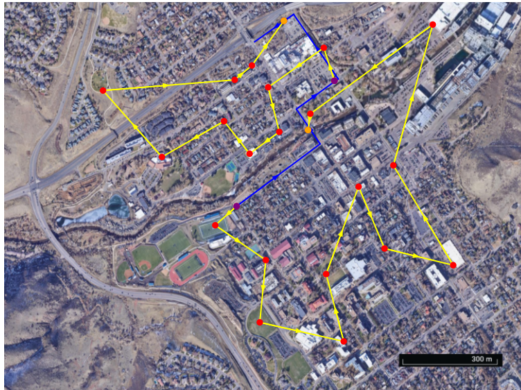
Fig. 12. Drone path generated using f -MINLP approach for a case study in an urban environment. The red circles are drone waypoints, the purple circles are drone launch locations, and the orange circles are drone landing points. The yellow line shows the path of the drone and the blue line shows the path of the GV.
